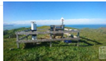
GPS site in Cape Campbell that recorded land movements from the earthquake
