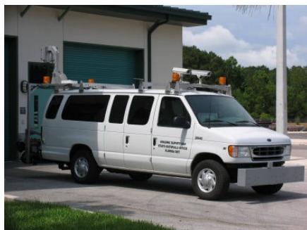
Figure 1: an example of a full width laser set up, fitted with cameras
