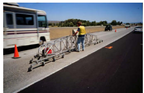
Figure 1: an example of a full width laser set up, fitted with cameras
