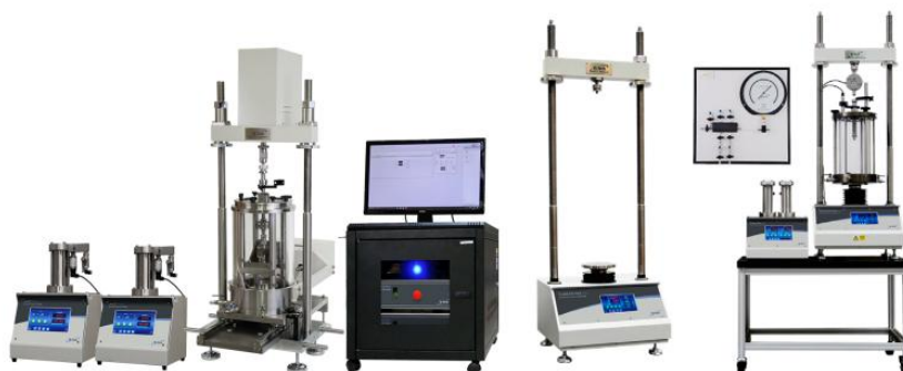
Dynamic Cyclic Simple Shear System with Confining Pressure
